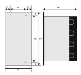
MODULE PANEL MOUNTING: B=85 \* H=175 \* D=110mm
